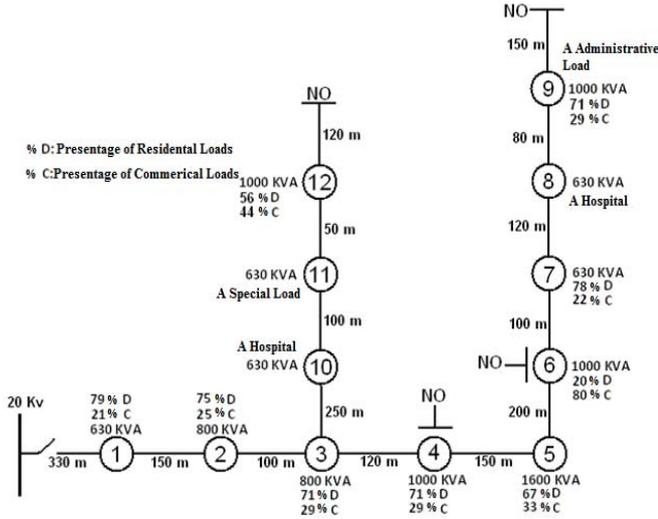
Fig. 4. The test system, a real part of the distribution system, located in the East of Tehran, Iran.
