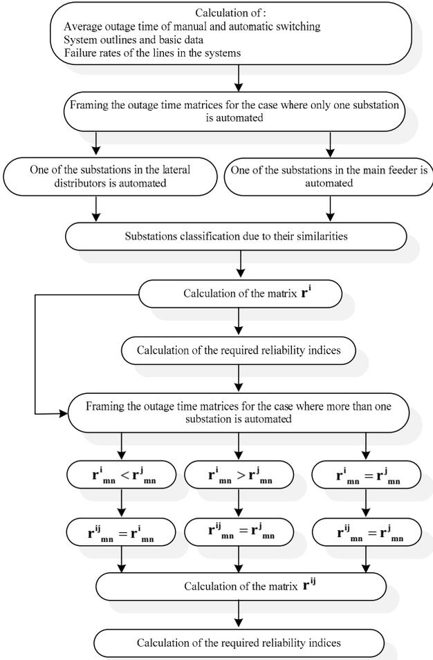
Fig. 1. The flowchart associated with the proposed methodology on the calculation of outage time
