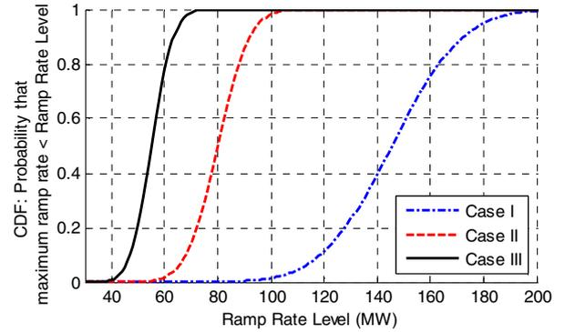
Figure 4. Cumulative distribution of the maximum ramping requirement of the system for 6 hours scheduling period and 40% PV penetration level.
