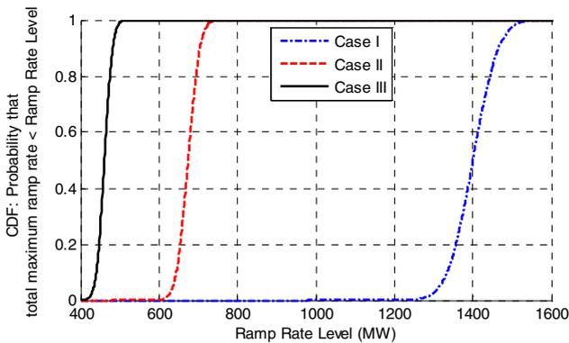
Figure 3. Cumulative distribution of the system total maximum ramping requirement for 6 hours scheduling period and 40% PV penetration level.
