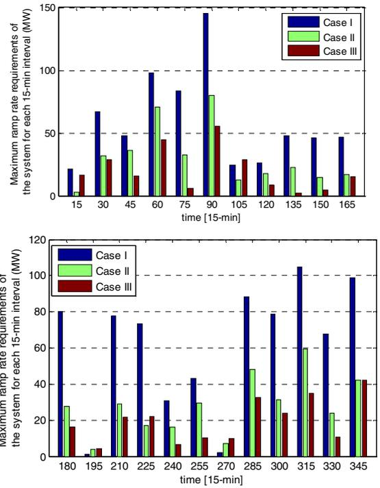
Figure 2. Expected value of the maximum ramping requirements of the system at each time interval  $RR_{max}(t)$  for a 6 hours scheduling period with 15-min time interval and 40% PV penetration level.
