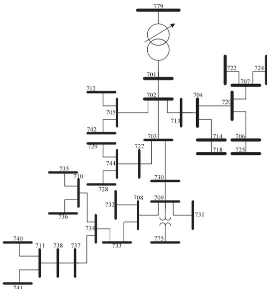
Fig. 3. The IEEE 37-bus test system under study.
