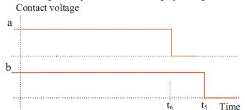
Fig. 3. ‘a’ and ‘b’ contacts transition during opening
