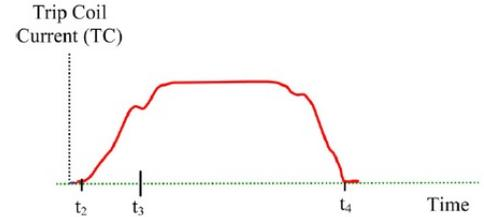
Fig. 2. Trip coil current during opening
