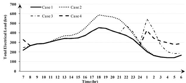
Fig. 7. Load profiles of various charging control algorithms (45%).
