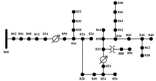
Fig. 3. Single line diagram of the IEEE 34 node test system.
