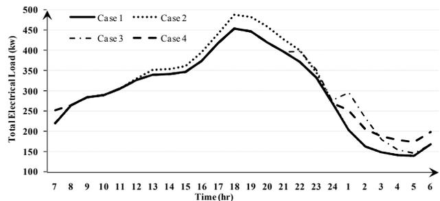
Fig. 5. Load profiles of various charging control algorithms (11.3%).
