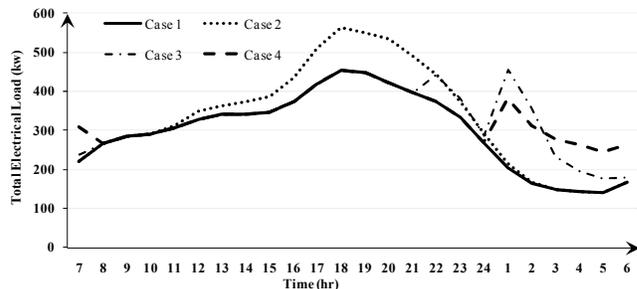
Fig. 6. Load profiles of various charging control algorithms (35%).
