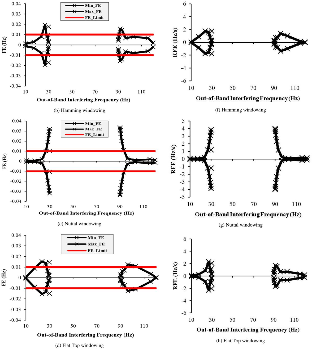
Fig. 3. Out-of-band frequency test performance of PMU at 60Hz using different windowing algorithms: Frequency Errors (FE) (a)-(d); Rate of Change of Frequency Errors (e)-(h).
