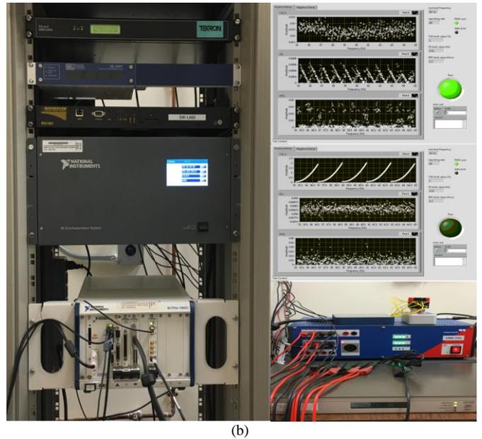
Fig. 1. Calibration platform for PMU testing.
