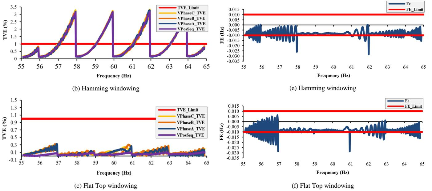
Fig. 2. Frequency ramp test performance of PMU algorithms using different windowing algorithms: voltage TVE (a)-(c) and frequency error (d)-(f).
