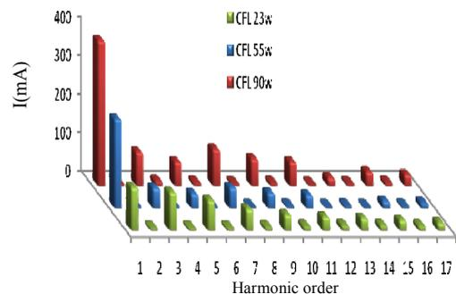
Figure 4. Experimental result of CFLs (harmonic content).
