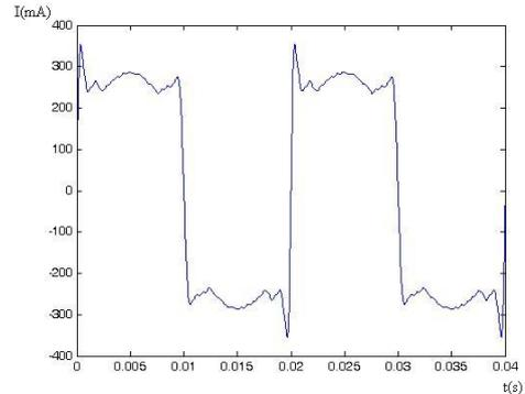
Figure 1. CFL current wave form (23 W).
