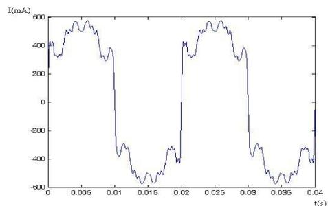
Figure 3. CFL current wave form (90 W).
