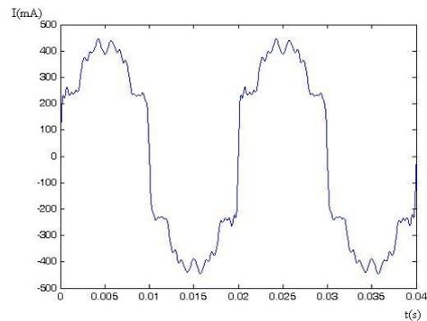
Figure 2. CFL current wave form (55 W).
